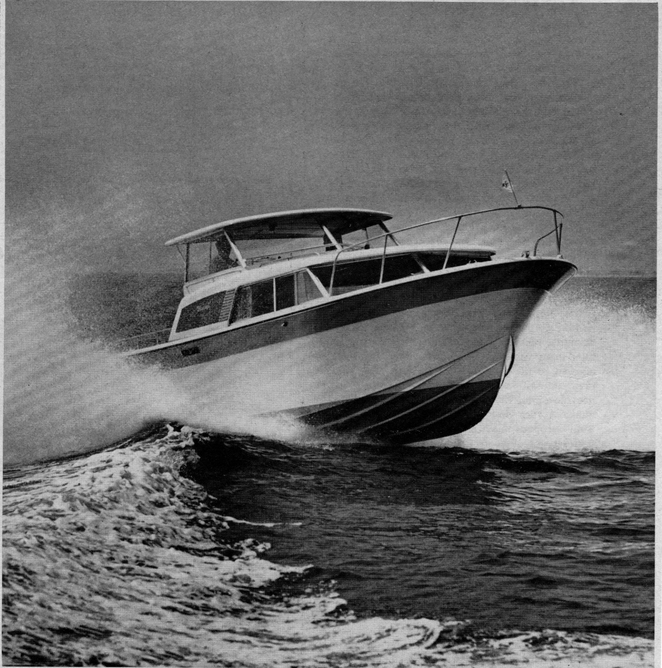
Tollycraft 27-footer combines generous flare, ample freeboard, and modified deep-V hull to produce soft, dry ride.
