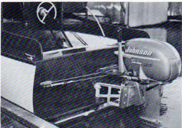
Transom step, and motor mount on our 20 Foot VACATIONER
