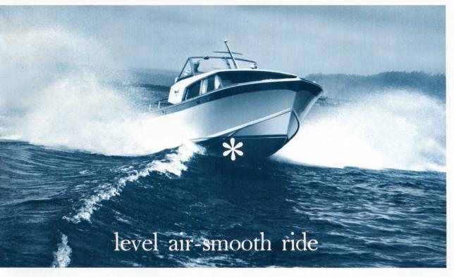
This remarkable new hull design is primarily a modified deep vee type featuring longitudinal planing stabilizers (L.P.S.) scientifically placed to achieve maximum directional stability.
