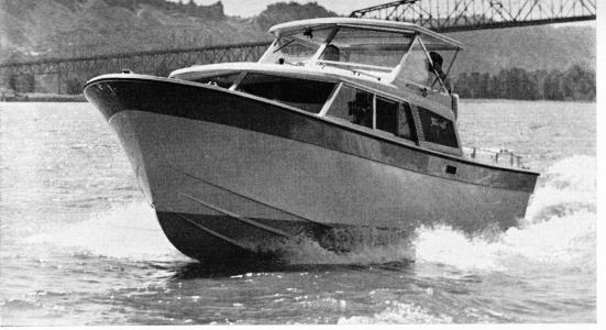
The 23-foot cabin cruiser got its power from a 185-horse OMC outdrive that's rated to handle up to
