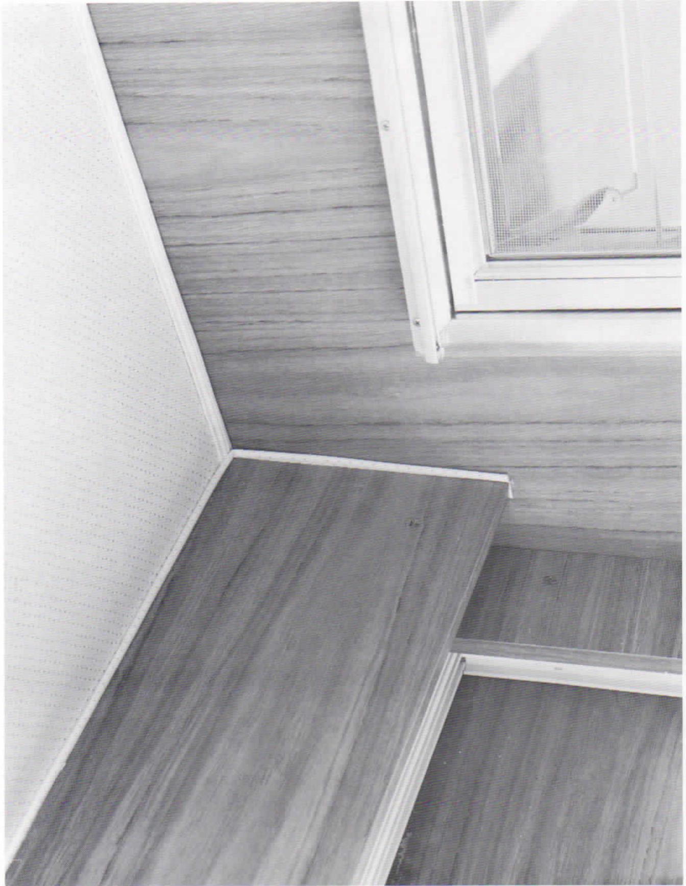
Perforated vinyl headliner material enhances the professional finish on the interior of a Tolly.
