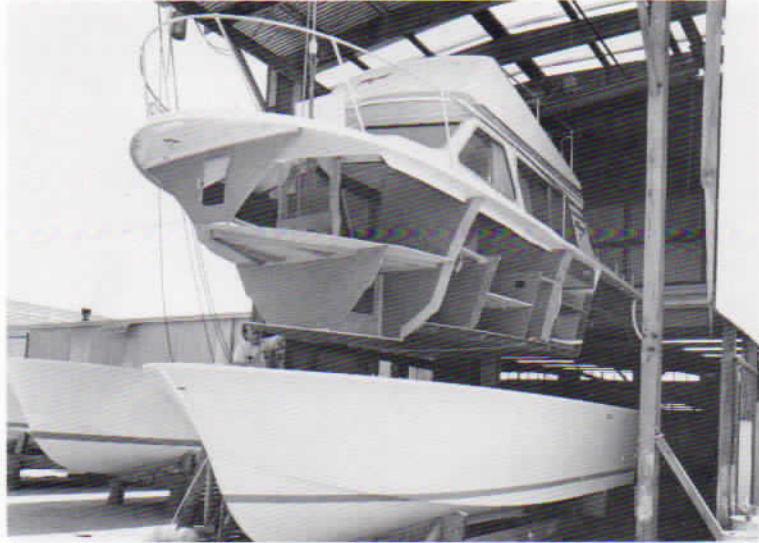
The cabin liner and deck are raised above a 26' Sedan hull.
