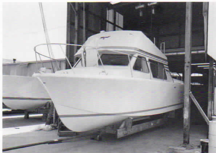
The cabin is fiberglassed to the hull.
