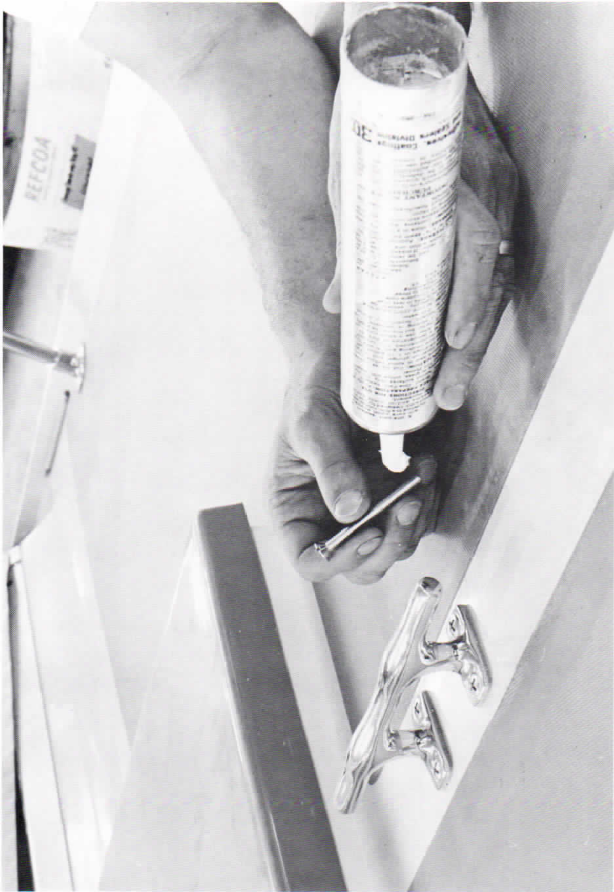
Bolts on all deck fittings are coated with marine sealant to help prevent leaks.
