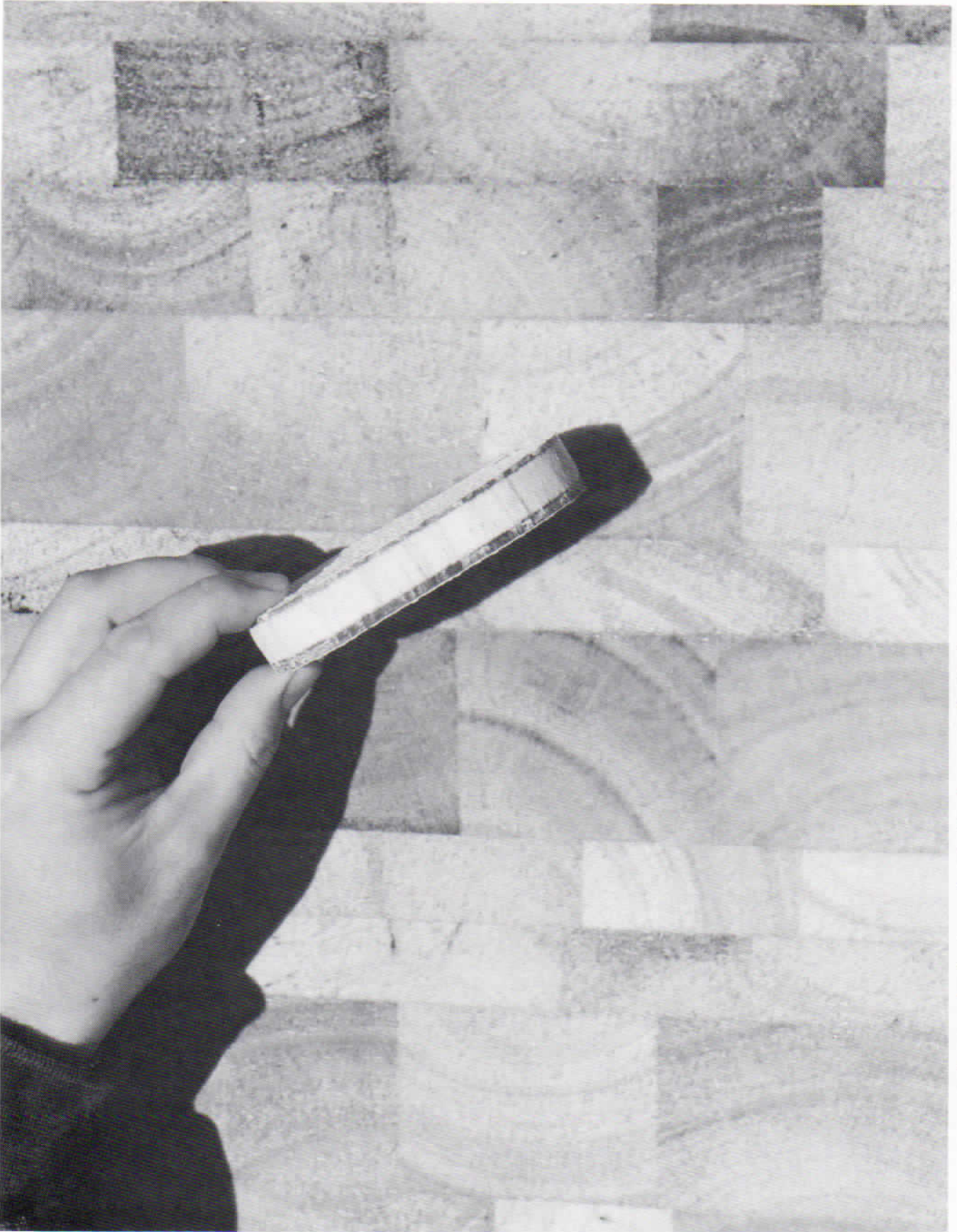
End grained Balsa is sandwiched in between double layers of fiberglass on all decks and cabin tops for strength, rigidity and insulation.
