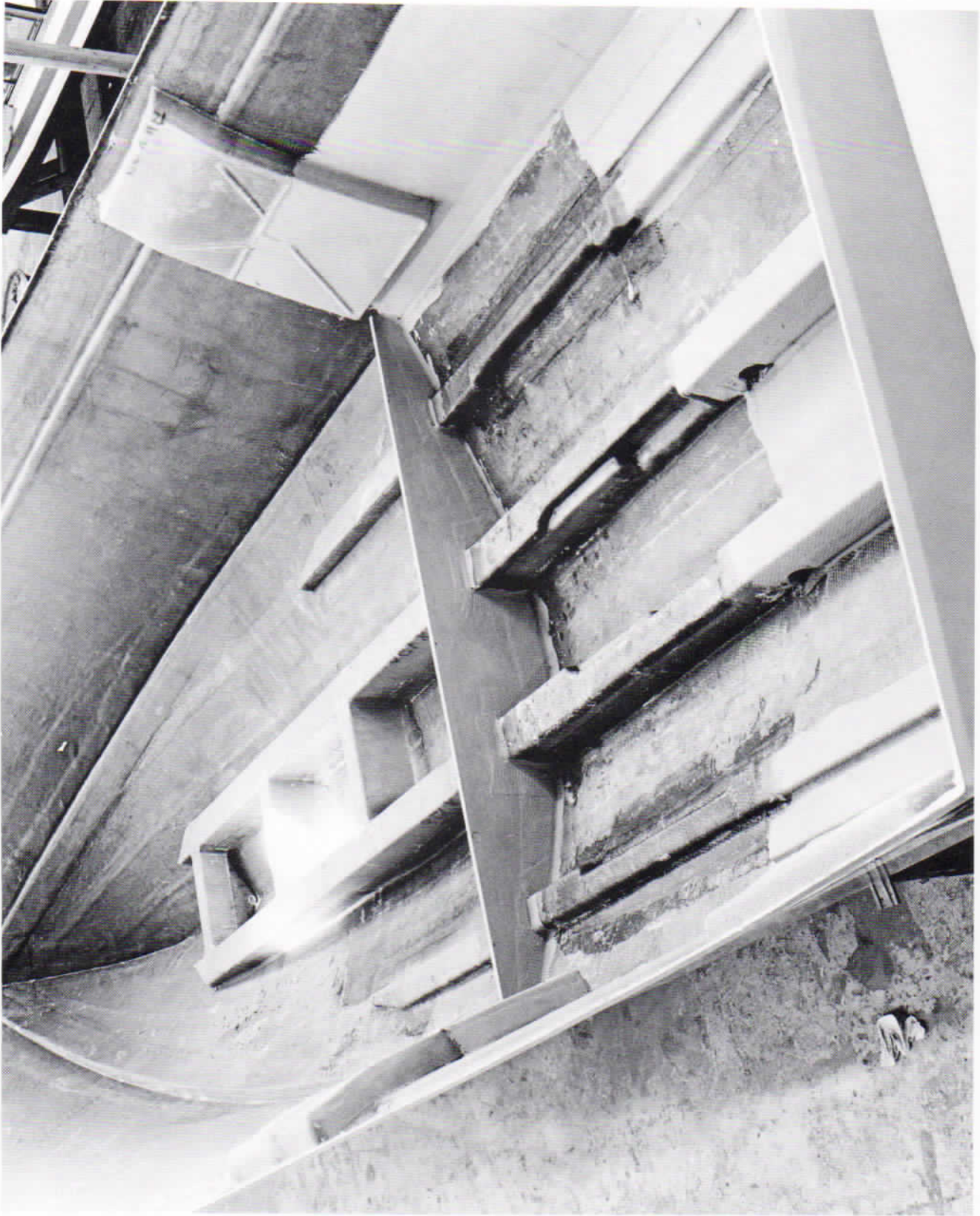
Engine stringers and longitudinals are molded fiberglass, permanently bonded to the hull.
